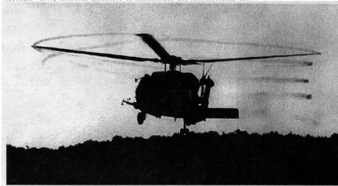
Figure 1.5 Flow visualization of tip vortices in hover due to natural condensation 6
